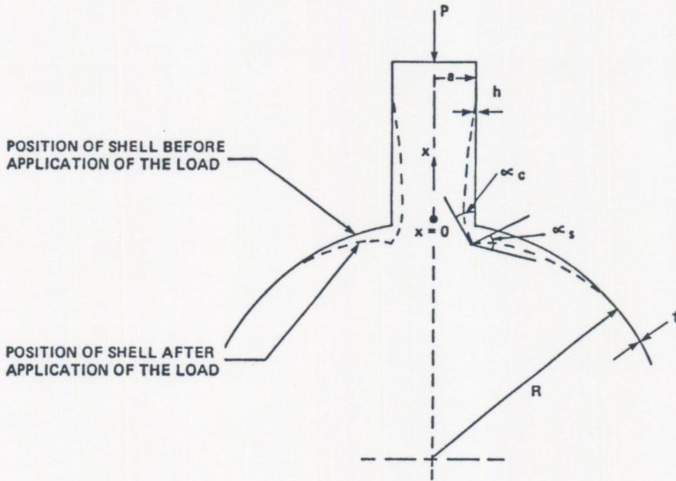
FIG. 2 POSITION OF SHELL BEFORE AND AFTER APPLICATION OF RADIAL LOAD
