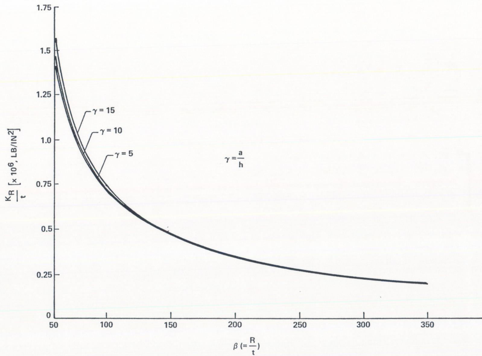
FIG. 6 GRAPH FOR RADIAL SPRING CONSTANTS FOR  $\rho = 10.0$
