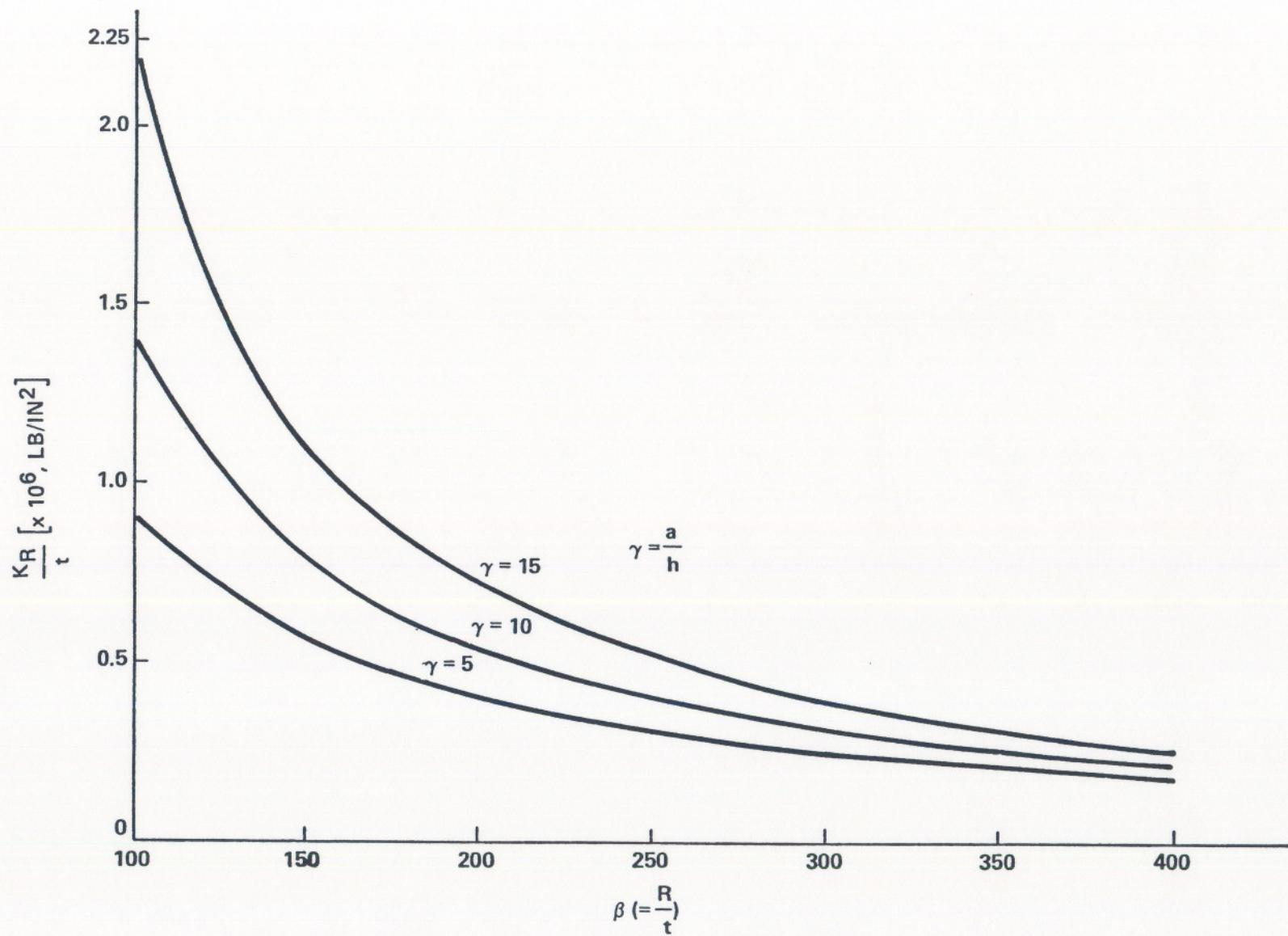
FIG. 4 GRAPH FOR RADIAL SPRING CONSTANTS FOR  $\rho = 2.0$
