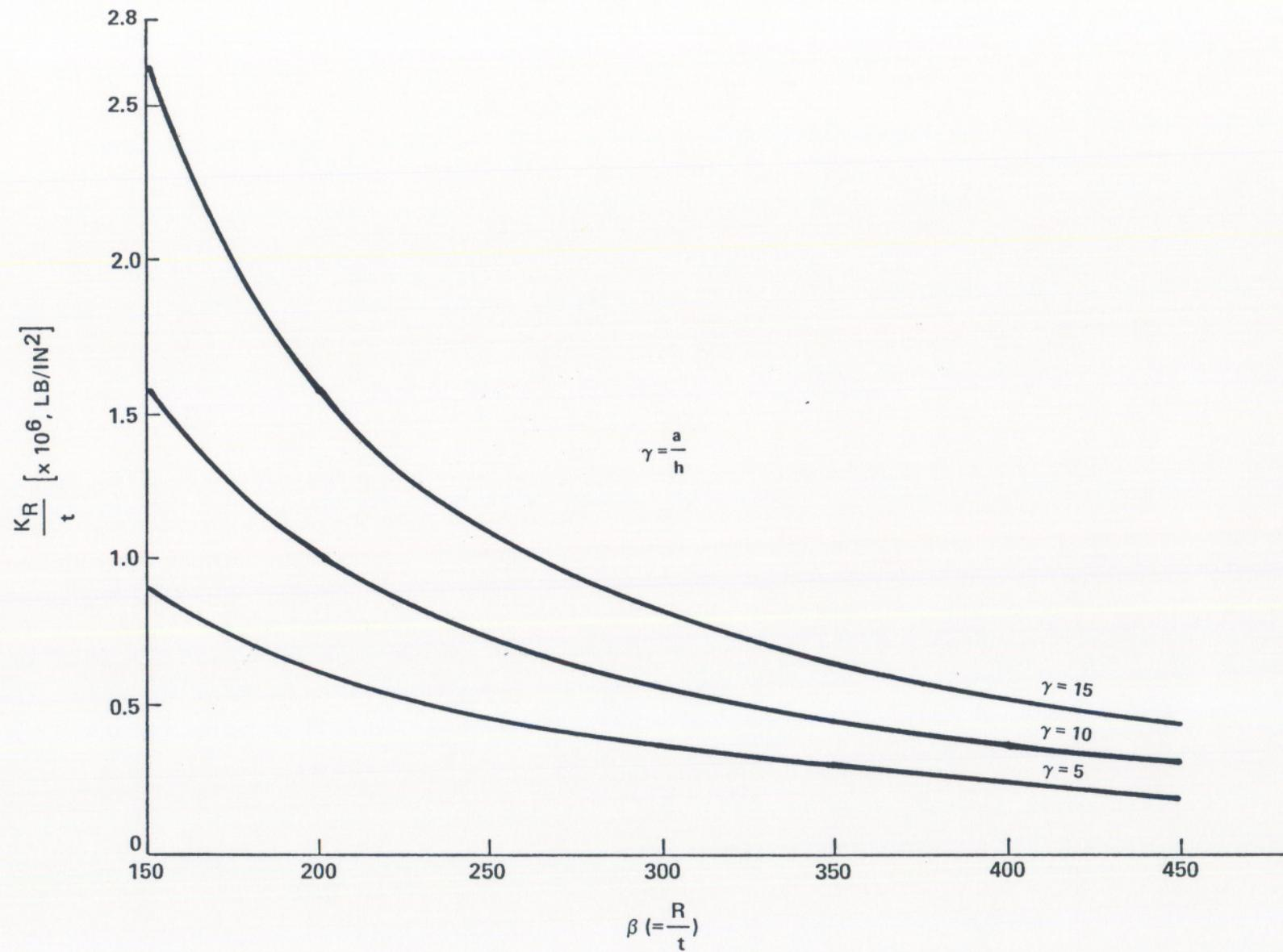
FIG. 3 GRAPH FOR RADIAL SPRING CONSTANTS FOR  $\rho = 1.0$
