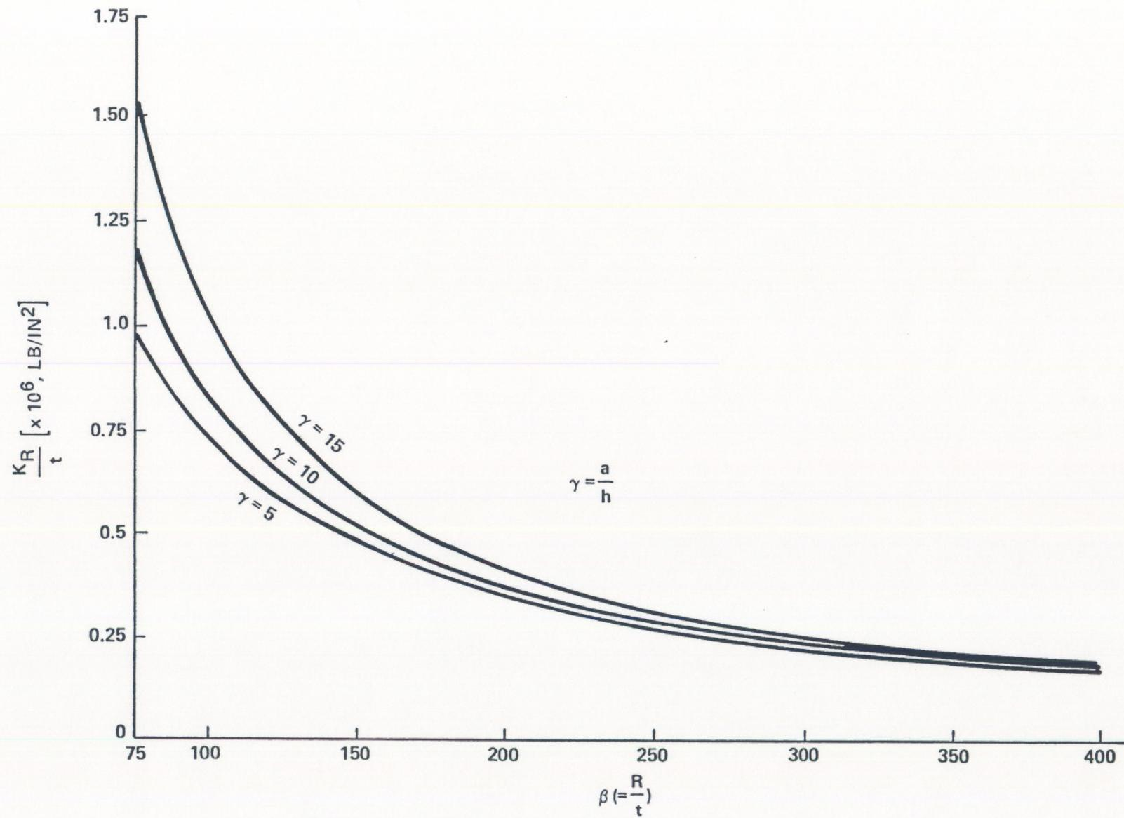
FIG. 5 GRAPH FOR RADIAL SPRING CONSTANTS FOR  $\rho = 4.0$
