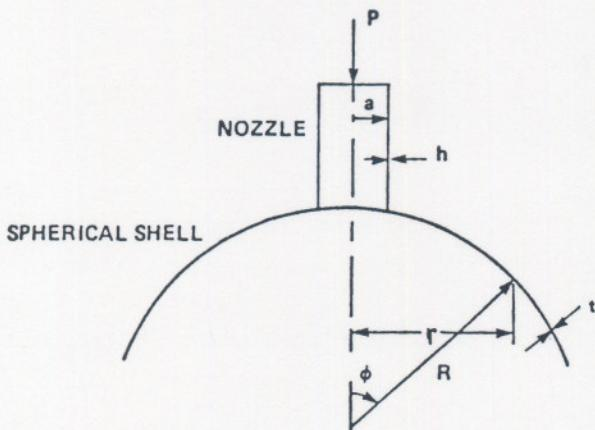
FIG. 1 SPHERICAL SHELL SUBJECTED TO A RADIAL LOAD ACTING UPON A NOZZLE
